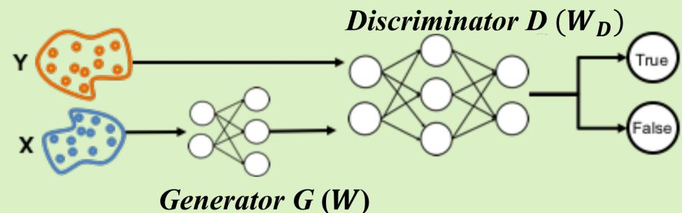
$\mathbf{D}: L_D(W_D|W) = -\sum_{i=1}^n \log P_{W_D}(source = True|Wx_i) - \sum_{i=1}^n \log P_{W_D}(source = False|Wy_i)$   $\mathbf{G}: L_G(W|W_D) = -\sum_{i=1}^n \log P_{W_D}(source = False|Wx_i) - \sum_{i=1}^n \log P_{W_D}(source = True|Wy_i)$
